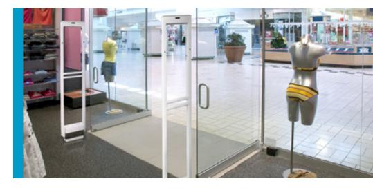
enhance store performance and increase conversion rates. Integrating directional traffic information with EAS alarm events allows the sensors to discern between inbound and outbound traffic, virtually eliminating unintended alarms triggered by shoppers carrying protected merchandise near the pedestals. Peoplecounting sensors also enable a "poweron-demand" feature that puts the system into low-power standby mode during periods of low or no traffic activity to reduce power consumption up to 90%.
